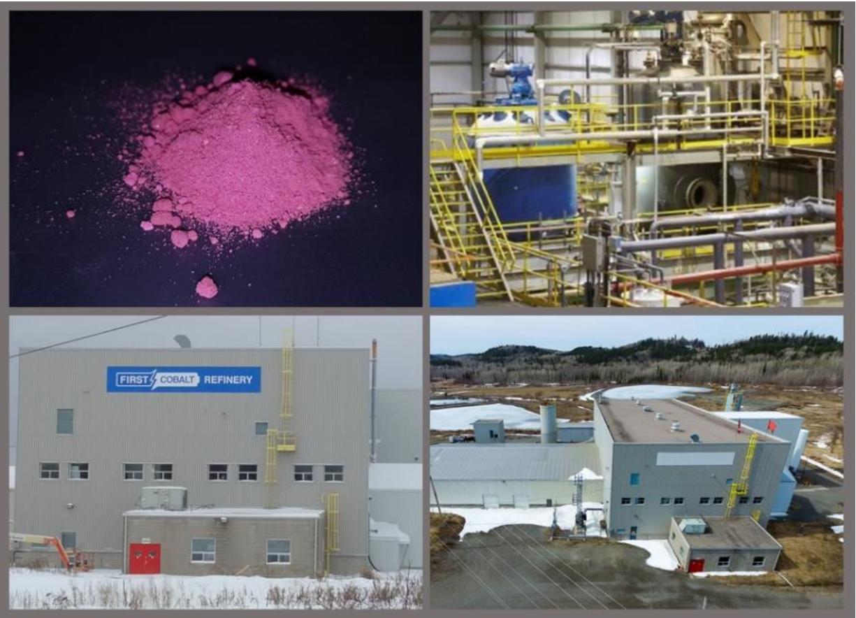
Image 1. Top left to right, cobalt sulfate produced using the First Cobalt Refinery flowsheet; current autoclave circuit. Bottom left to right, external and areal images of the facility.
