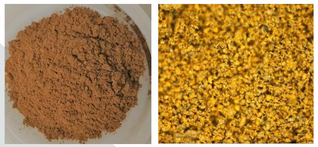
Plate 1 - AVL's V<sub>2</sub>O<sub>5</sub> product (right hand side image of product under microscope)
