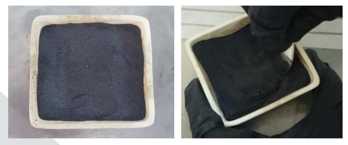
Plate 2 - Magnetic concentrate prior to roasting (left) and post roasting (right)
