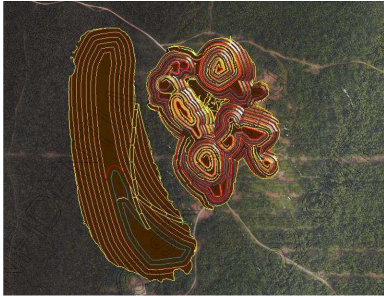
Figure 13 Busai Final Pit and Dump Design
