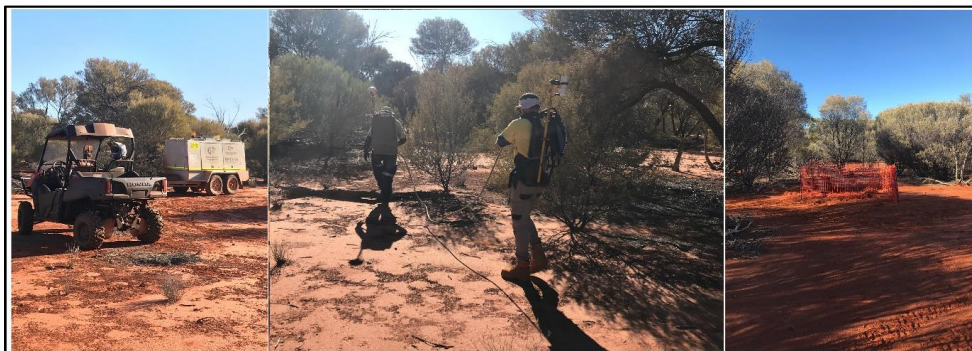
Figure 1: SAM survey includes the generation of an electric source from a transmitter (left) that is channelled into the ground (right) and detected at surface (centre)
