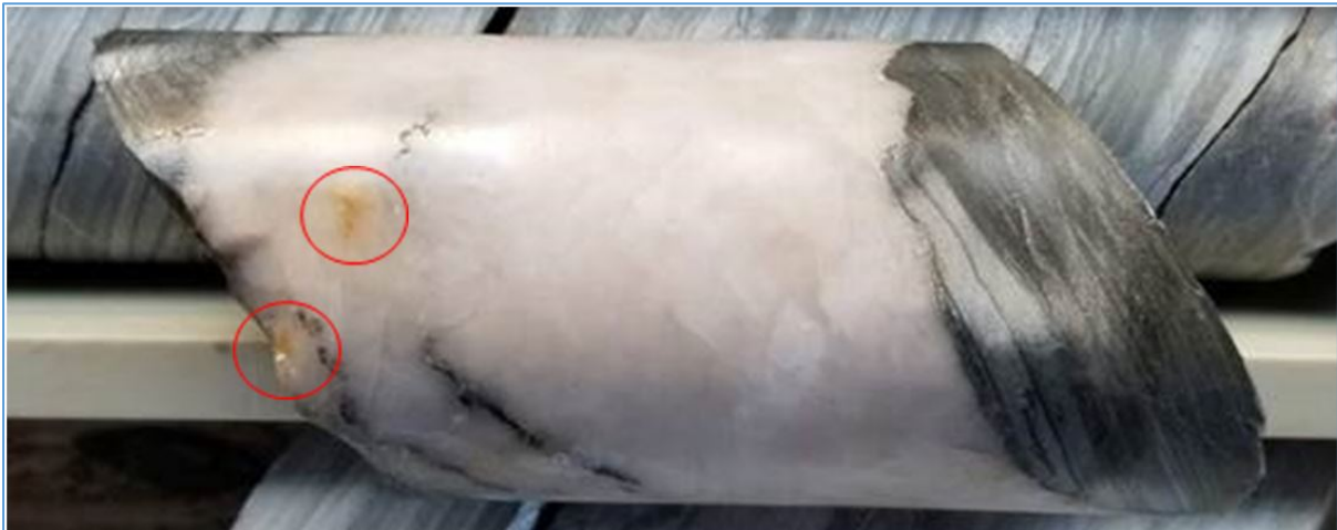
Figure 6 – Photo of core sample in TDD002A (from 251.9 to 252.0 m) illustrating massive white shallow dipping quartz vein with visible gold (circled)
