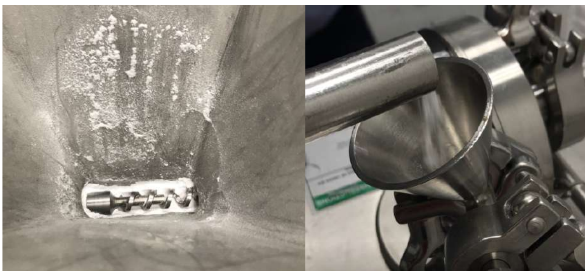
Figure 4: Lithium Carbonate in the Hopper of Jet Mill (L) and Entering the Jet Mill (R)
