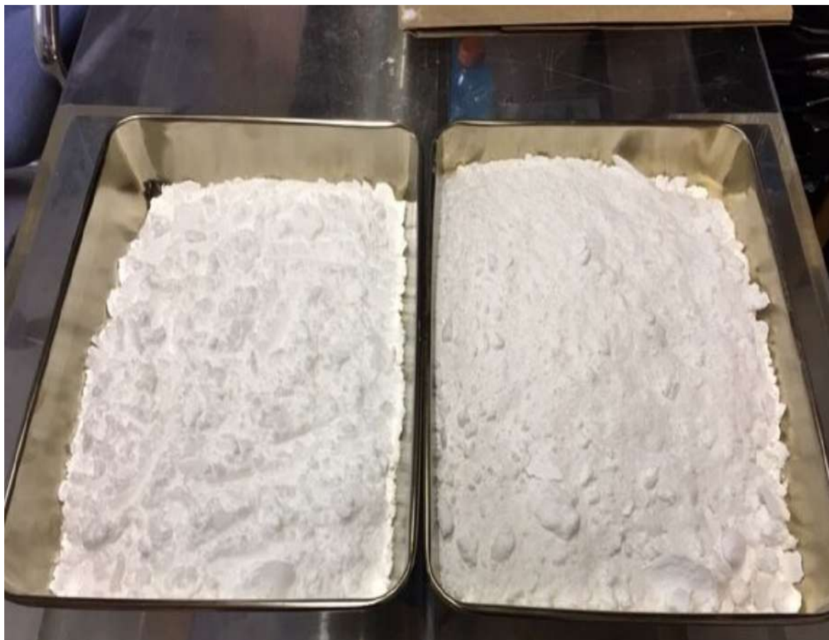
Figure 3: Lithium Carbonate Drying in Trays at the Southwest Technologies' Laboratory
