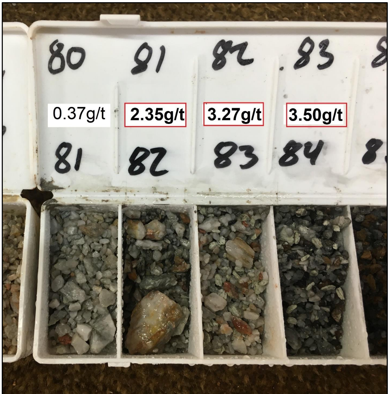
Figure 2: Mineralised interval in KWGLRC02 showing quartz vein, 3m @ 3.04g/t
