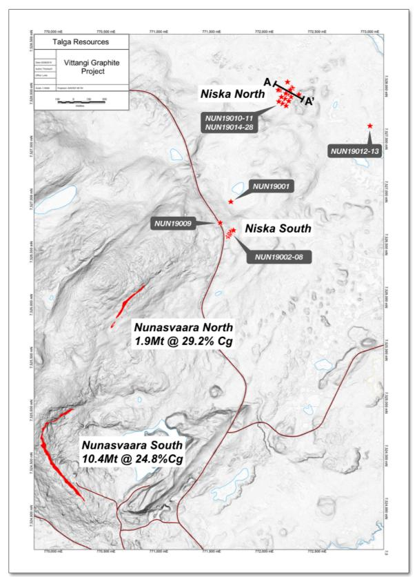
**Figure 3** Topography image of the Vittangi Graphite Project showing the drillhole locations at Niska North and South with current graphite resources at Nunasvaara North and South.
