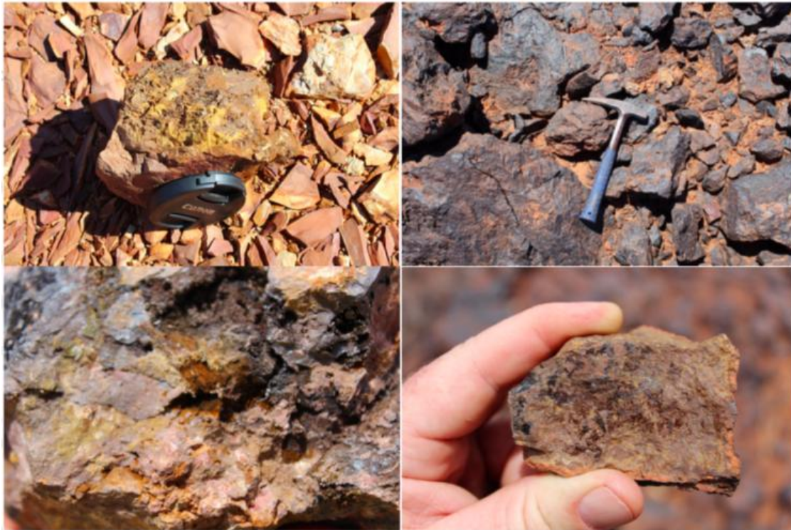
Rock chips from reconnaissance mapping: top right – ferruginous sedimentary breccia; top left - strongly manganeseiferous, fine grained sediment; Bottom left and right – fine iron oxides, possibly after sulphides, within fine grained sedimentary units.
