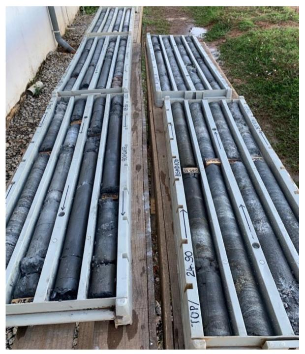
Figure 3: Diamond core for BSMD106 of the Mahela Prospect showing significant saprolitic graphite mineralization.
