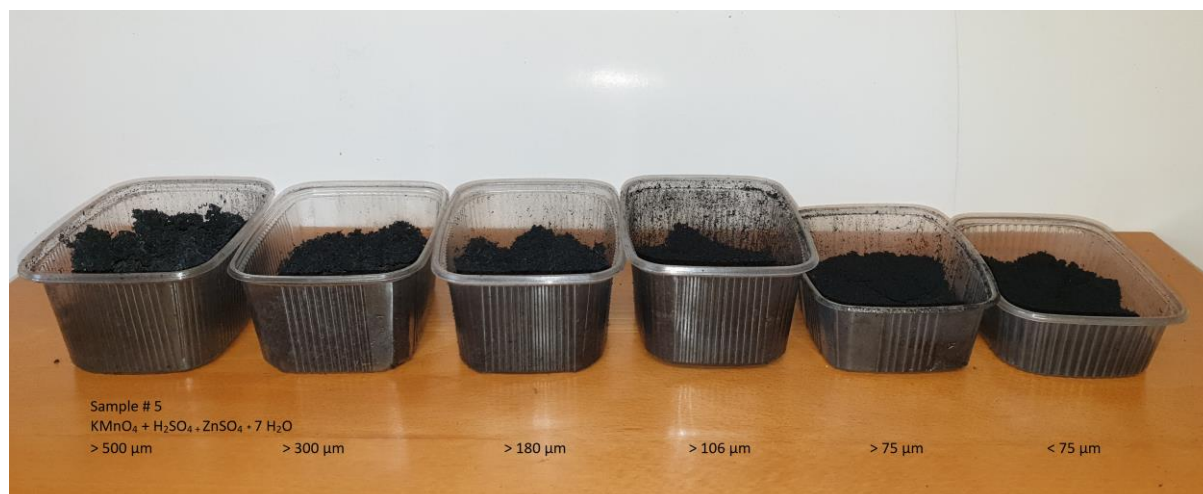
Image 1 - Photos of BEM product from NGS following expandability test work
