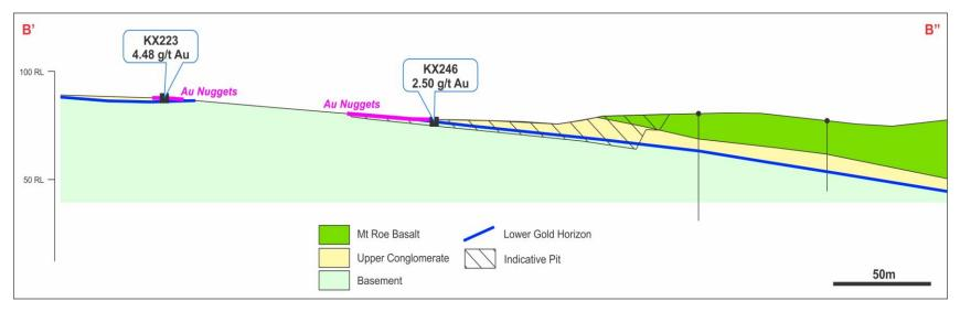
Example cross-section showing the bulk sample results and target gold horizon at Purdy's Reward, with an indicative pit geometry hatched.
