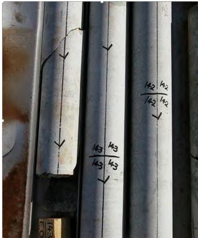
Figure 9.2 Example of diamond core with various degrees of fracturing, and the impact it has on the quality of the orientation mark-up
