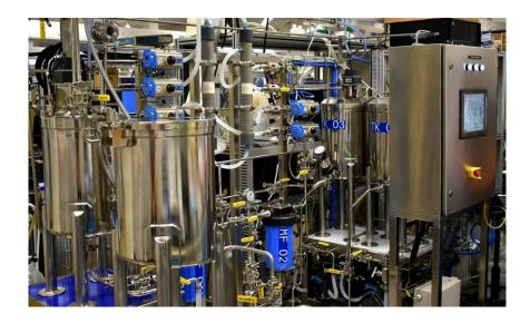
IMAGE 1) FO de-watering/liquid concentration system delivered by De.mem
