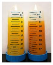
IMAGE 3) Beverage concentration on milk and fruit juice – beverage (feed) on left vs. concentrate on right
