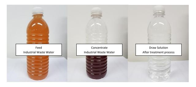
IMAGE 2) Industrial waste water - Feed vs. concentrate and draw solution from De.mem FO
