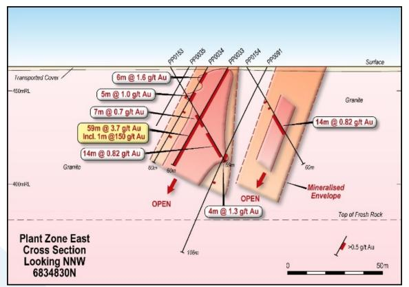
Figure 4 – Plant Zone Cross Section
