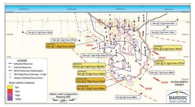
Figure 2. Alpha Lode long section looking 340°
