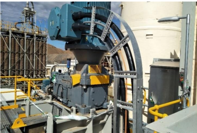
Figure 4: UFG Mill #1 with Spiral concentrator in background
