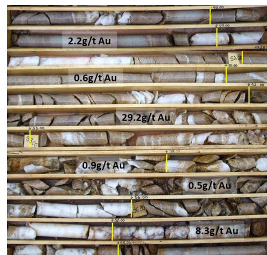
Figure 6: Core from DDH-02, 48-58m depth averaging 4.3g/t Au
