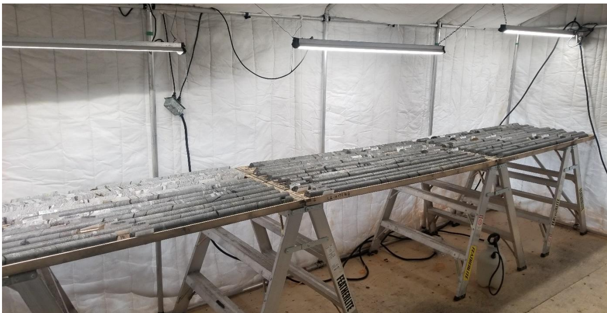
Figure 4: Drill core of DDH LR19-09 which intersected the Graphitic Carheil Zone over an extensive thickness of 70.0m at an average grade of 17.1% Cg at a depth from 9.0m to 79.0m.
