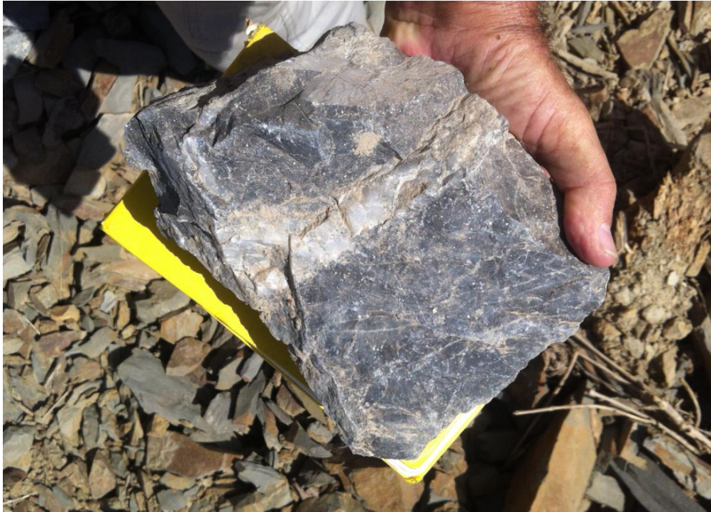
Plate 4: BouBou/Bourdala Permit – Bourdala/TD Artisanal Workings. Gold bearing quartz-carbonate vein in silicified-carbonate-sulphide altered meta-sediment.
