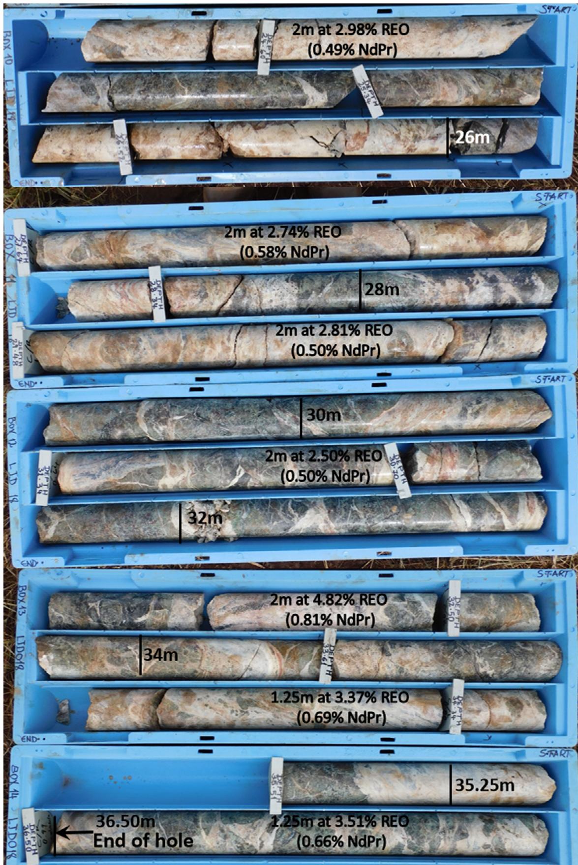
Above: Lower portion of diamond core hole LJD018: 14.5m at 3.22% REO including 0.58% NdPr to end of hole in fresh rock carbonatite (cream)-fenite (grey) breccia. Trays are 1m long. Core is PQ3 diameter (83mm).
