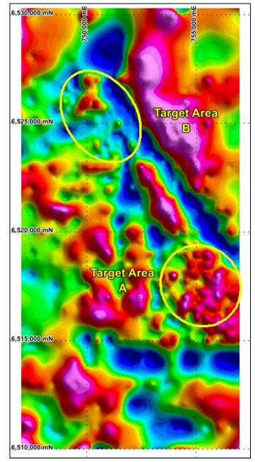
Figure 2. Residual gravity image over Tasman's Pernatty Project (EL 6137). Red/magenta colours are areas of stronger residual gravity, generally indicating areas likely to be underlain by denser rocks. Also shown are Target Areas A and B where a number of relatively shallow potential IOCG systems have been modelled (GDA 94, MGA Zone 53).
