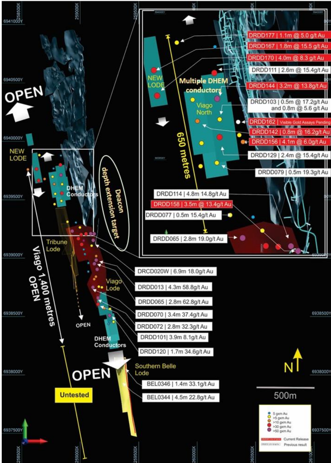
Figure 7: Plan view of Viago Lode showing recent northern discovery & southern extensions and recently defined DHEM plates. Only the northern extension has been included in this resource upgrade and drilling is continuing at Viago Main and to the south. The Viago Lode now extends for over 1,400 metres and remains open.
