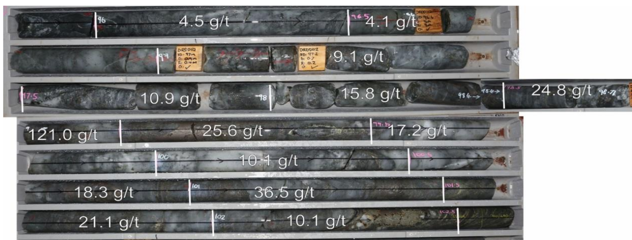
Figure 2: Drill core from Tribune South diamond core hole DRDD112 high-grade mineralization associated with ~15% semi massive pyrrhotite, trace disseminated chalcopyrite and fine-grained visible gold. Interval assayed 6.5 m @ 22.2 g/t gold.
