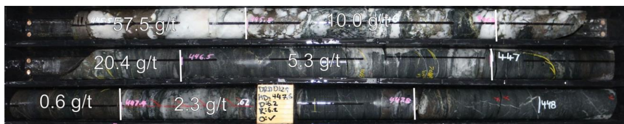
Figure 4: Viago North diamond core hole DRDD129 high-grade mineralization associated with ~15% semi massive pyrrhotite, trace disseminated chalcopyrite and fine-grained visible gold. Interval assayed 2.4 m @ 15.4 g/t gold.
