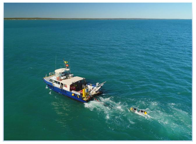
Image: The *Prowler* towing the airgun array during production operations
