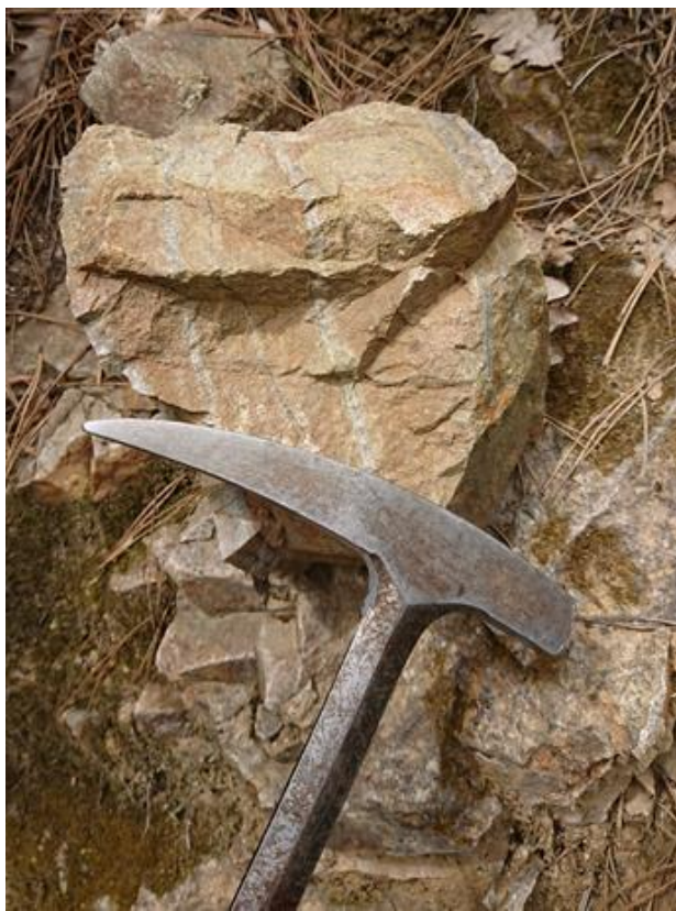
Figure 3 - Sheeted quartz veining within an Andesite stock. This type of veining may be indicative of the presence of a porphyry deposit
