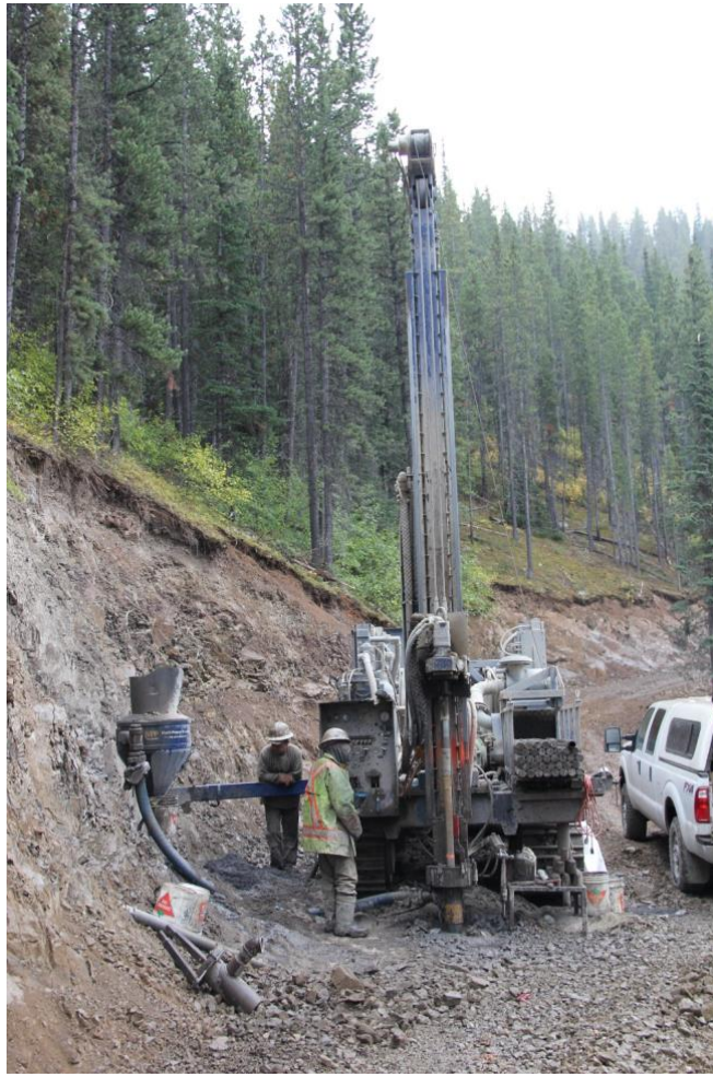
Figure 3: Percussion rig drilling at northern end of Oil Pad Trend
