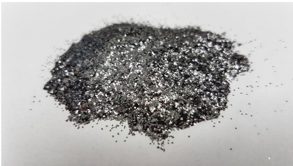
BEM jumbo flake produced by BGRIMM (China)
