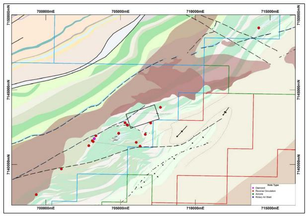
Figure 1. DD and RC Drilling conducted at the Morck Well Project during Q2, 2019.
