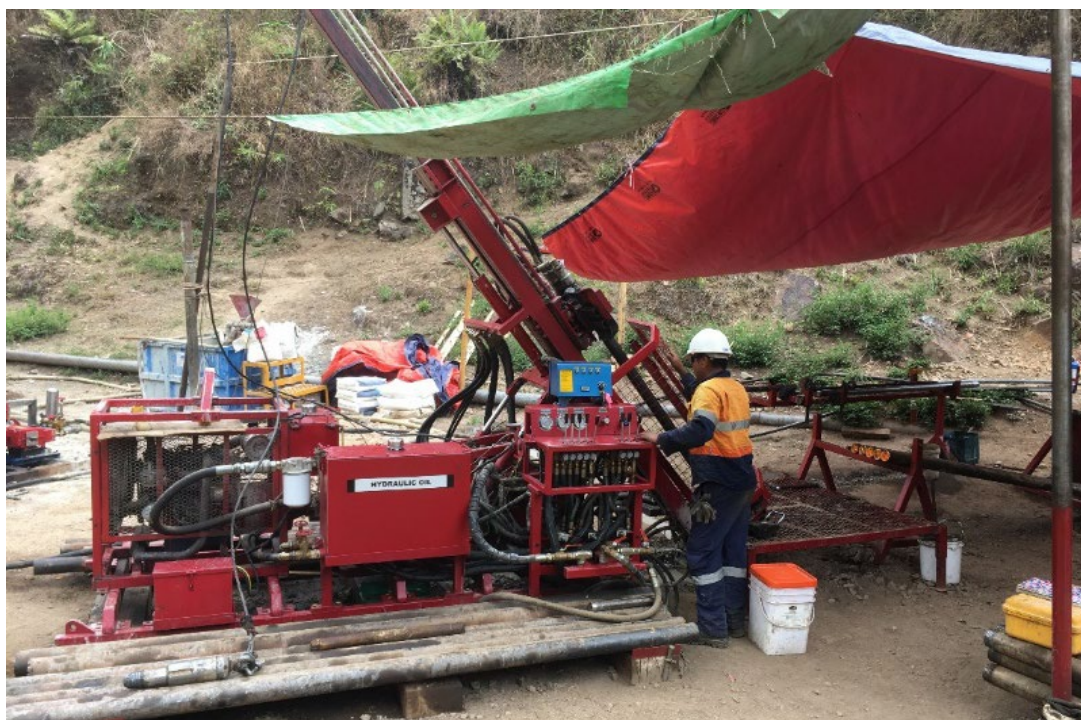
Figure 2. Shan North discovery hole BWDD030, being drilled by the man portable drill rig in the Bawdwin North village.
