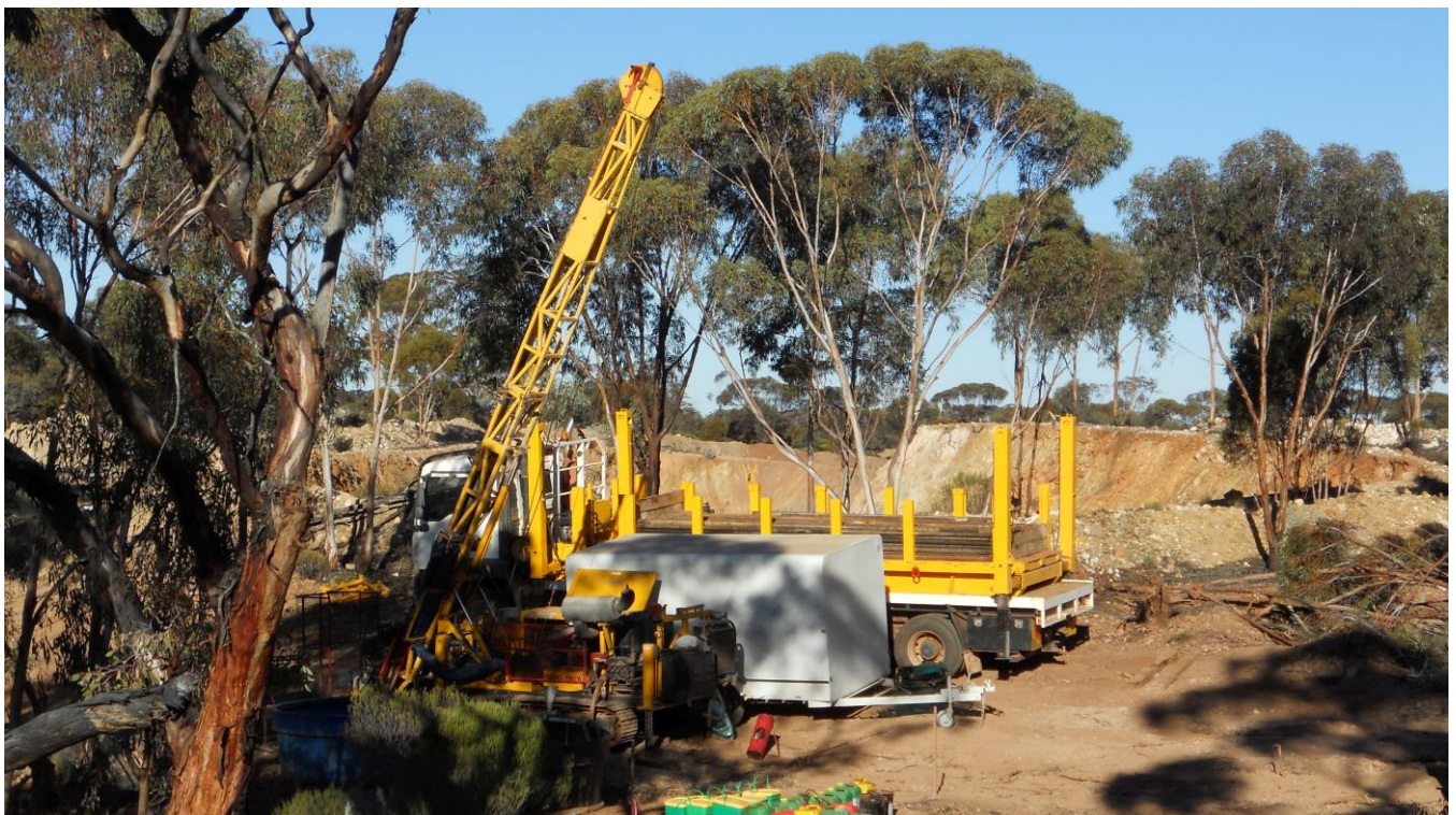
Figure 1. Topdrive Drilling Australia track-mounted diamond core rig setup and drilling at Munda Gold Project, Widgiemooltha WA.
