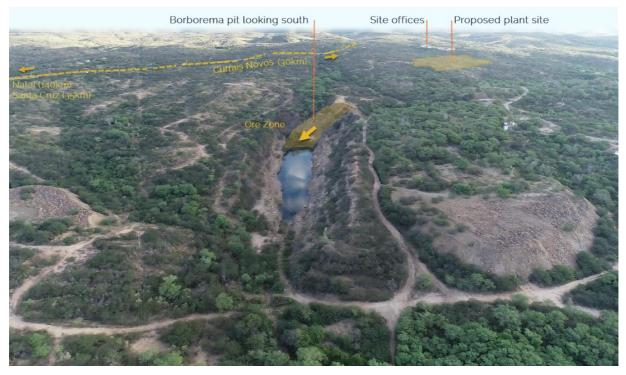
Figure 2. View to the south over Borborema project site showing gold mineralisation exposed in the pit and proximity of infrastructure. Transmission line to the left of the pit links with main power grid crossing the Borborema leases.
