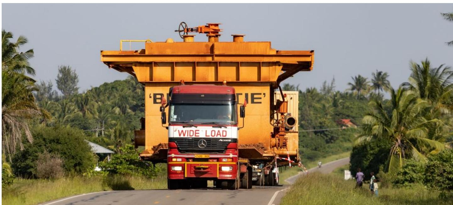
Moving the collection hopper during the transition of mining operations to the South Dune orebody
