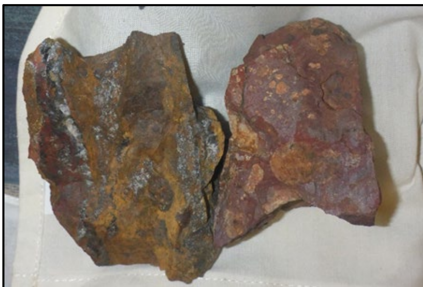
Figure 5: Oxide breccia sample with 6.5% copper & 0.8 ppm gold (CWRK013)
