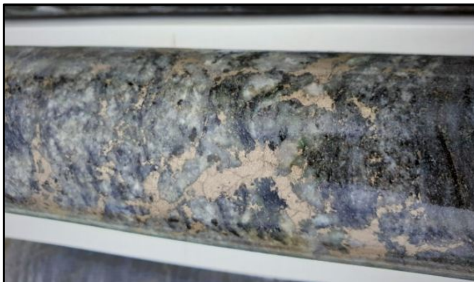
Figure 3: Sulphide stringers and veins with quartz in ER001 at 407m (field of view approximately 15cm across)
