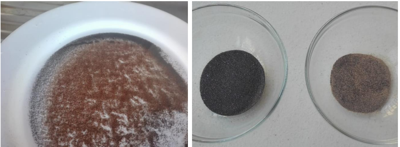
Figure 3 & 4: Photographs showing heavy mineral panned concentrate from soil samples (LHS) and magnetically separated fractions (RHS). The lower photograph is the non-magnetic fraction and shows significant visual rutile.
