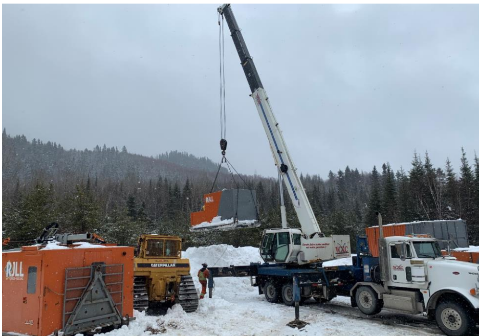
Figure 3: Diamond drill rig being set up at the first drill site at the Lac Rainy Graphite Project
