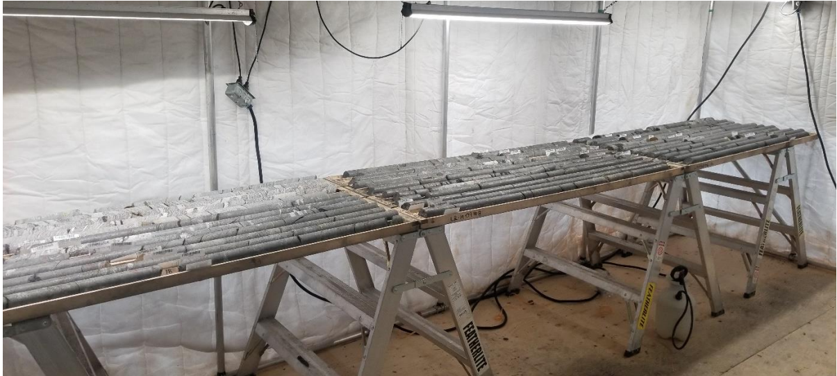
Figure 6: Drill core of DDH LR19-09 which intersected the Graphitic Carheil Zone over an extensive thickness of 70.0m at an average grade of 17.1% Cg at a depth from 9.0m to 79.0m.
