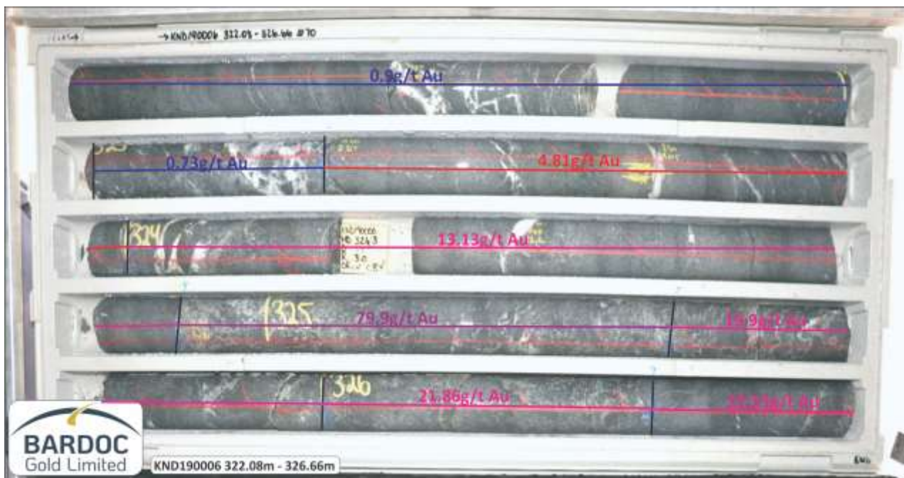
Figure 1. Annotated high-grade Blueys South Lode. Note the massive nature of the ore with even high-grade gold distribution. Quartz breccias are common for the hanging wall contact (323.3m).
