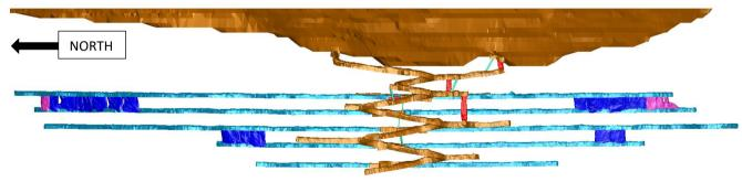
Figure 2: Bartons Underground Project Long Section showing mine development to date (blue).
