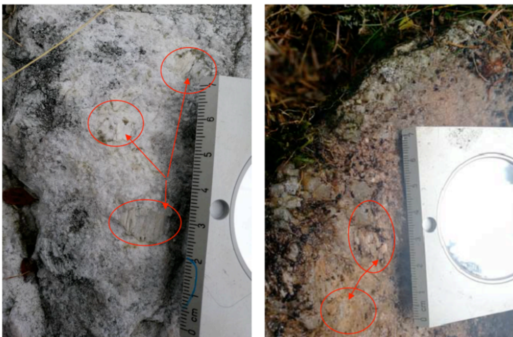
Figure 2 - - Field samples with spodumene (1 cm) crystals embedded into a qtz-feldspar matrix. Figure left sample 75001 3.39% Li 2 O, Figure right sample 75010 1.68% Li 2 O.
