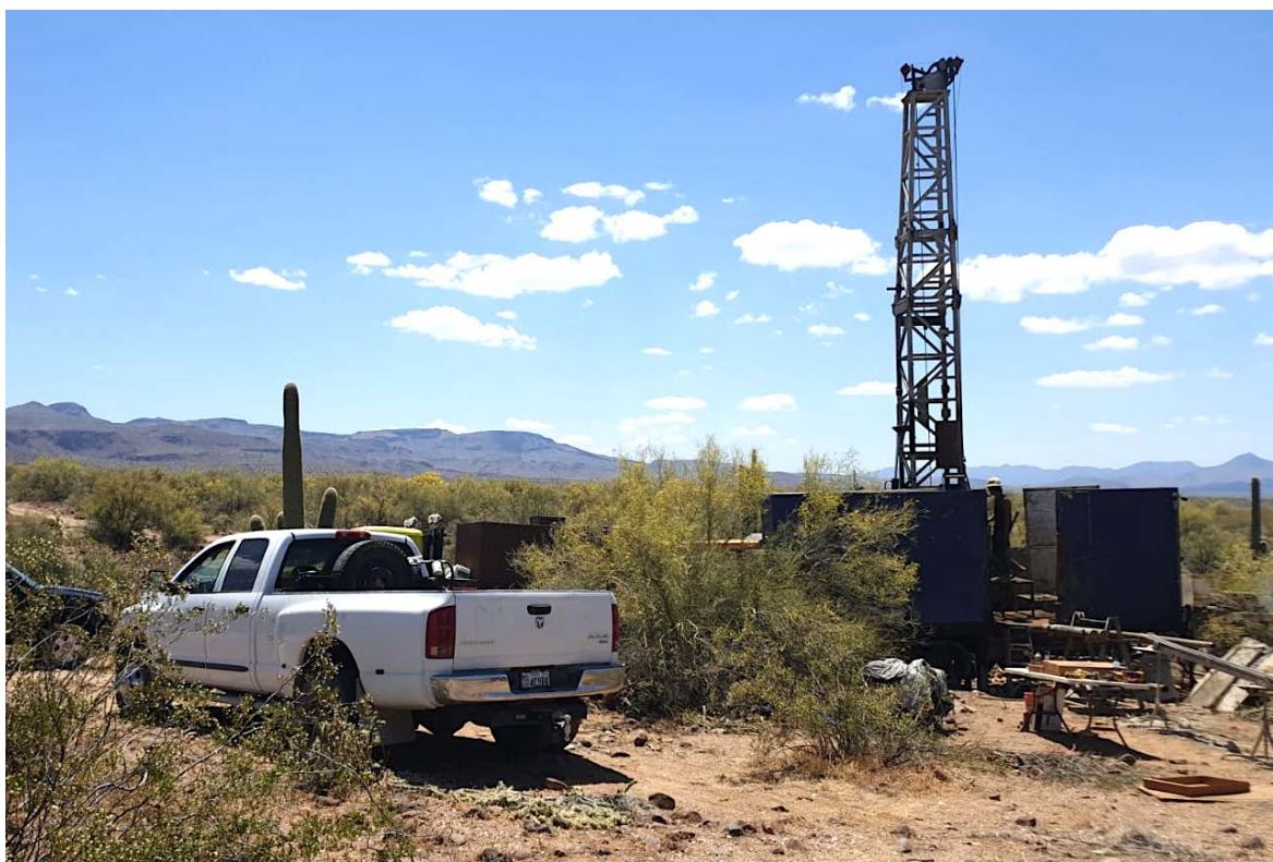
Image 3 (below) – Diamond drill rig on site at the Big Sandy Lithium project for the Company's 37 hole diamond drill program.
