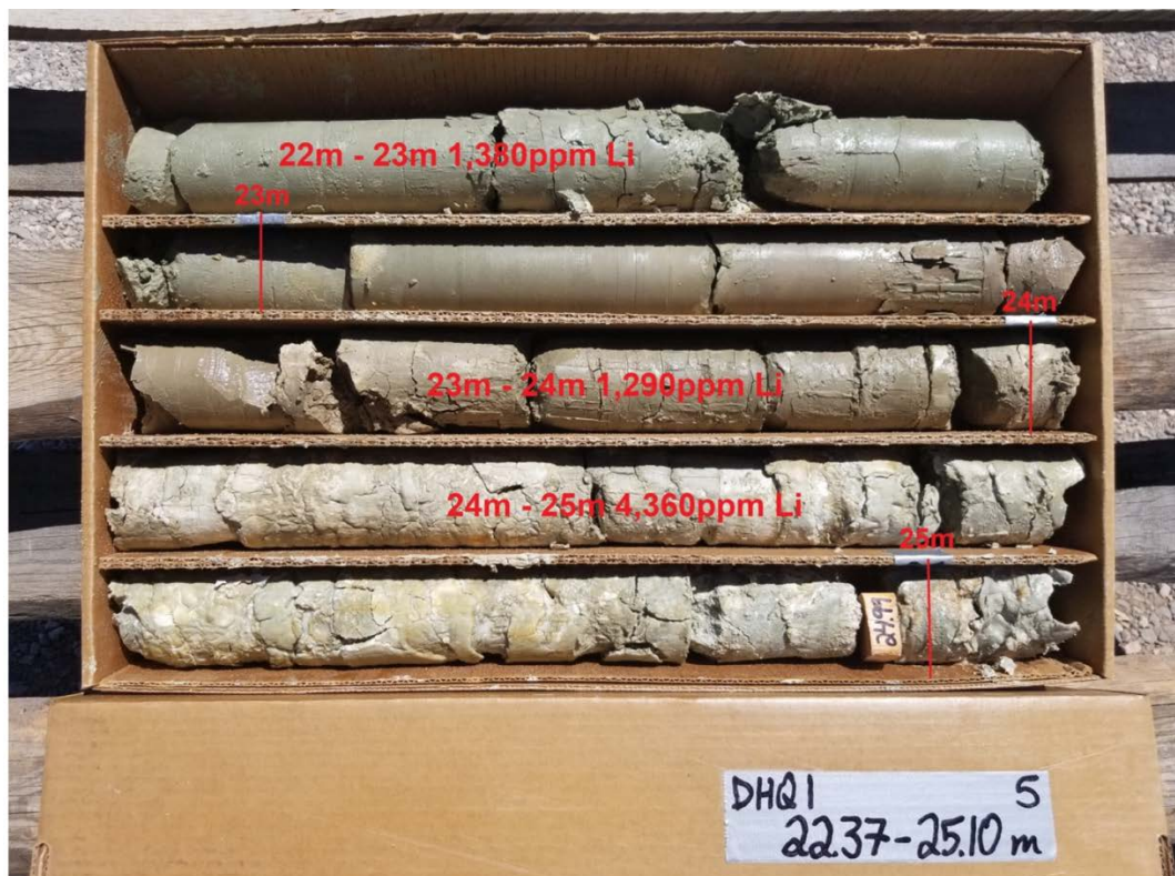
Images 4 & 5 (above and below) – Drill cores from Hawkstone’s 37 hole diamond drill program.
