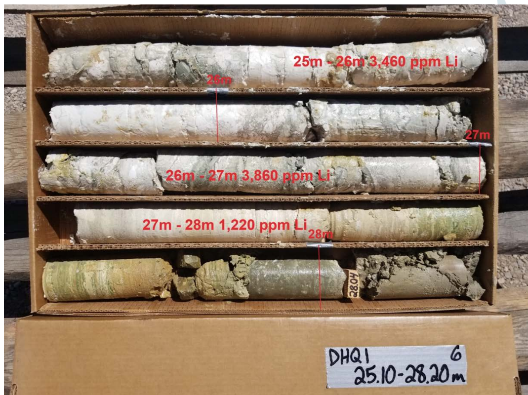
Images 4 & 5 (above and below) – Drill cores from Hawkstone’s 37 hole diamond drill program.
