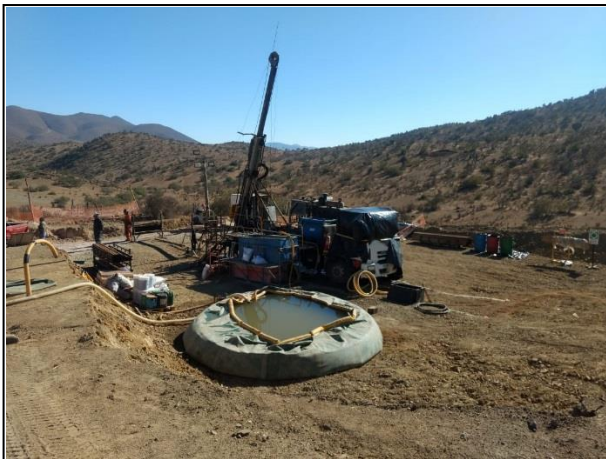
Photos 1 & 2: Diamond drill rig set up at Hole 1, Samuel Copper Project, the rig has now moved to hole 2.
