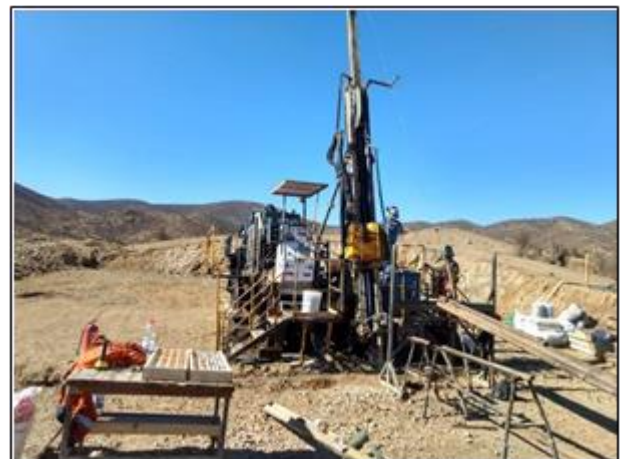
Photos 1 & 2: Diamond drill rig set up at Hole 1, Samuel Copper Project, the rig has now moved to hole 2.
