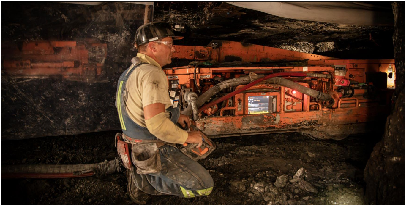
Figure 2: Underground continuous miner in operation at Poplar Grove
