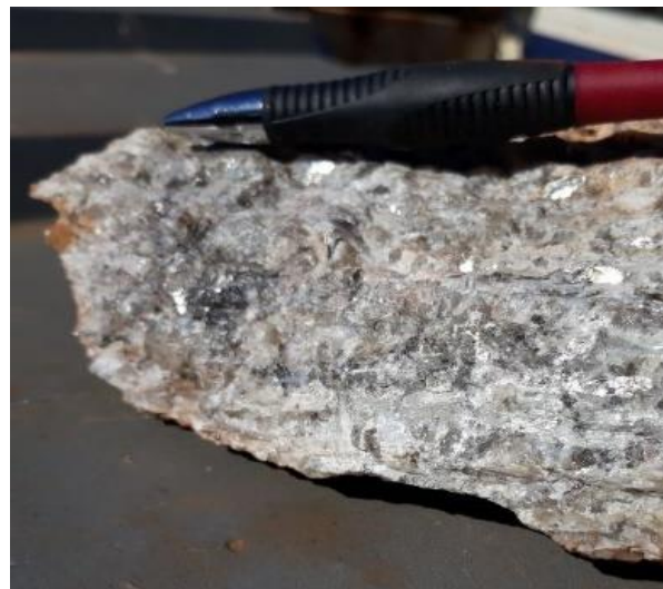
Figure 4: Shimmering elongate grey spodumene laths in pegmatite from Spodumene Target 2.
