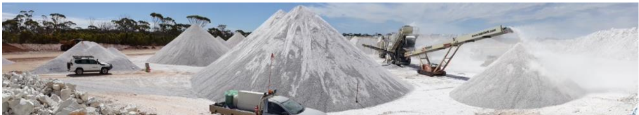
Figure 2: photo of pollucite being crushed and stockpiled.
