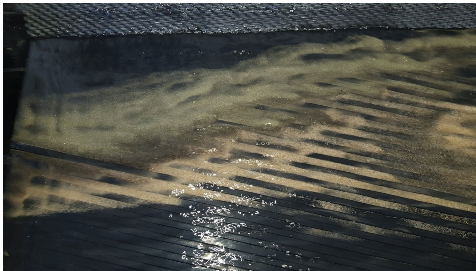
Figure 1 – precious metals and other heavy minerals being separated from host rock
