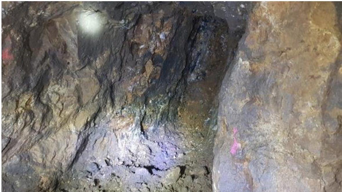
Figure 4 - the face of the Mystery Drive showing the extension of the vein before sidewall waste is removed
