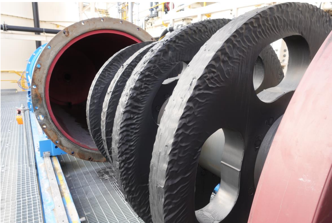
Figure 3 IsaMill™ undergoing internal inspection.
