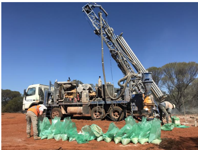
Figure 2: RC Drilling at Youanmi
