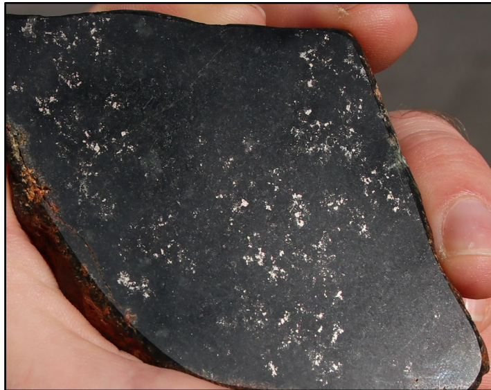
Figure 1. Quick Shears outcropping nickel-copper sulphide hand specimen
