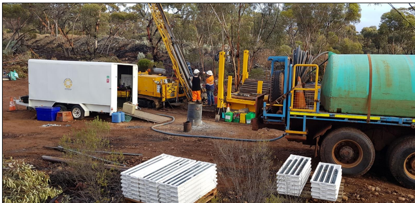
Figure 4. Topdrive Drilling Australia's diamond core rig at Munda with stacked core tray ready for collection at end of hole.
