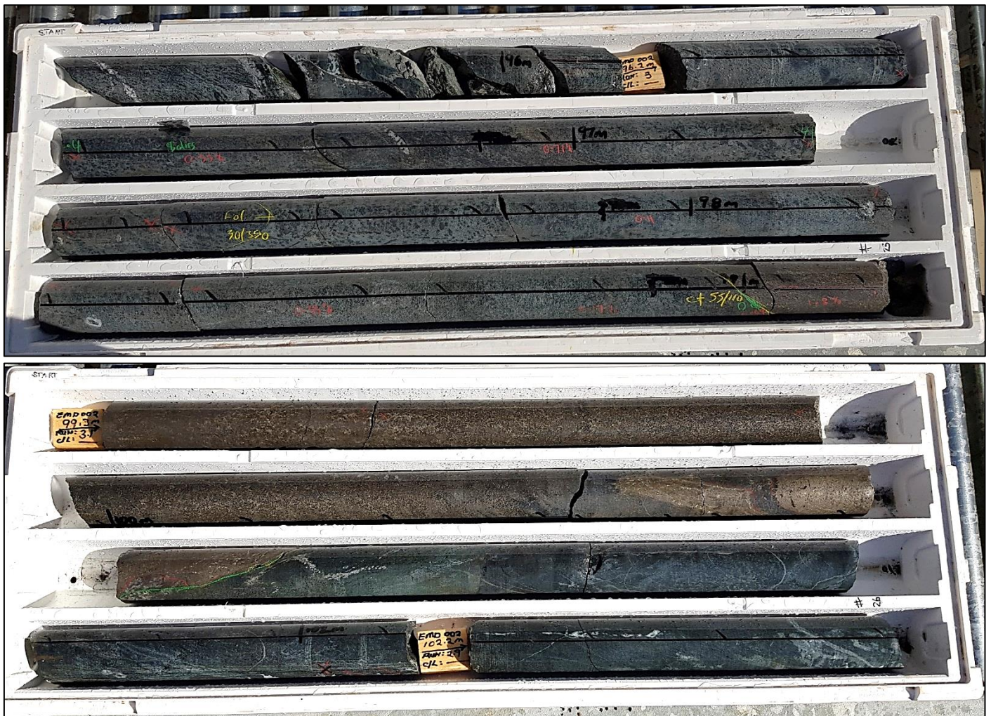
Figure 2. EMD002 intersection with disseminated sulphides from 93.0m-99.0m, matrix sulphide from 99.0m-100.6m, semi-massive sulphide on the basal contact from 100.6m -101.0m and stringer sulphides in the basalt contact zone from 101.0m-101.3m.
