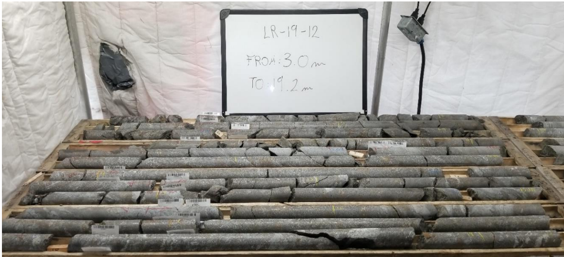
Figure 4: Semi-massive graphite flakes mineralisation intersected in DDH LR19-12 over a mineralised interval from 3.0m to 19.2m, contained within a wider zone of mineralisation.
