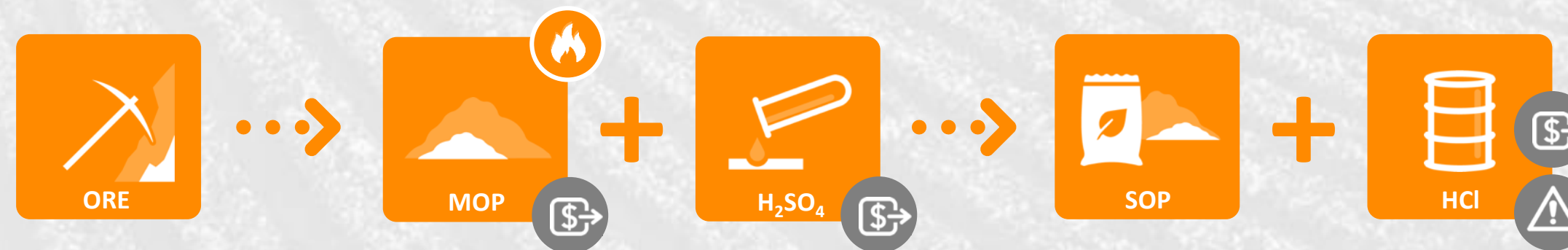
MANNHEIM PROCESS MOP heated to 600°C – 800°C in furnace
