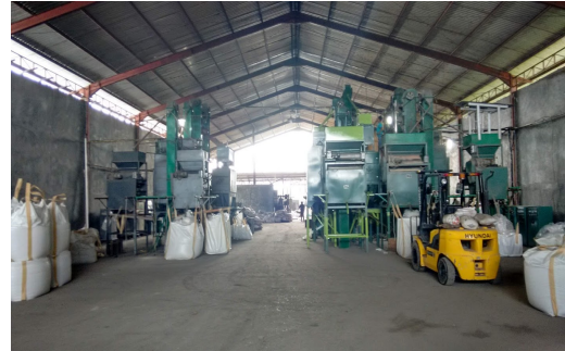
Figure 3(b): Electrostatic and Electromagnetic Separators Installed at the PTIM Plant
